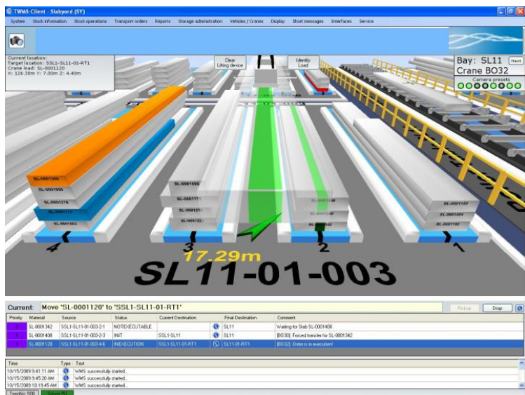
Typical crane driver view in a slab yard. Angle of view is changing depending on crane sensor data (position).
