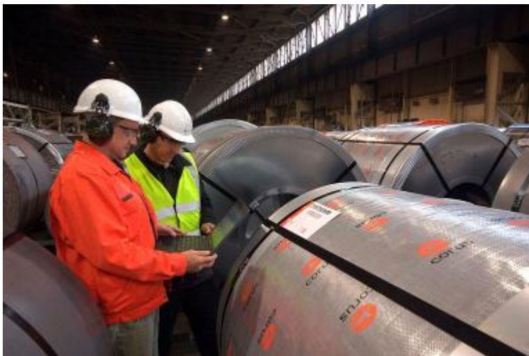
上图中为Corus带材厂在进行钢卷检测 © Corus Strip Products
